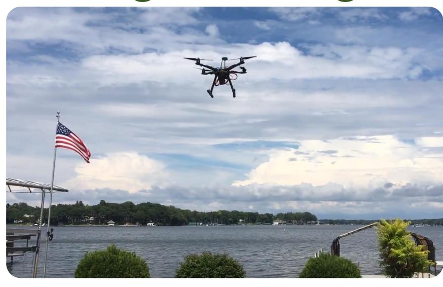
GPS and Optical Flow correction allow for the MAV to be very stable in indoor and outdoor environments. Outdoors, wind causes slight (~5cm) disturbances before the MAV detects enough movement to warrant a correction back to the desired position.
